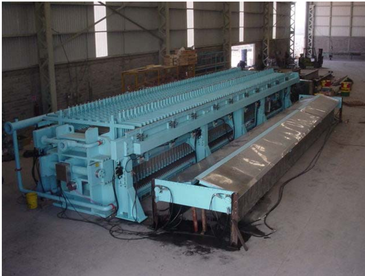
Filter and Drip Tray on Assembly Floor
