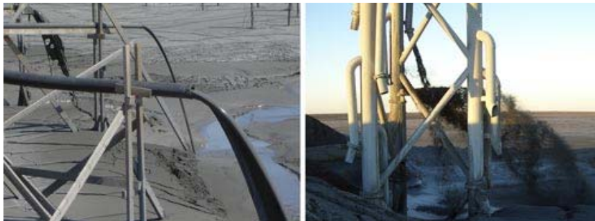
Surface thickened Thickened discharge at Kidd Creek, ON, Canada (left) and at Mt Keith, Western Australia (right)
